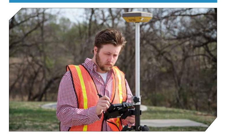
Land surveyors play an important role in the development and construction of buildings, roads and land. This crucial technical role is responsible for taking precise measurements with specialized equipment to determine property boundary lines and elevations. They also help construction crews ensure that building codes and zones are upheld. Land surveyors utilize GPS and GIS technology to collect information, create maps, mark property, and advise governments and businesses on planning
